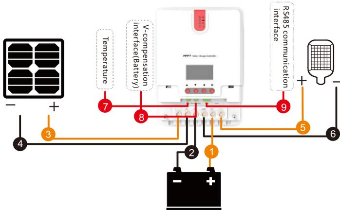
Fig. 2.3 Wiring sequence
