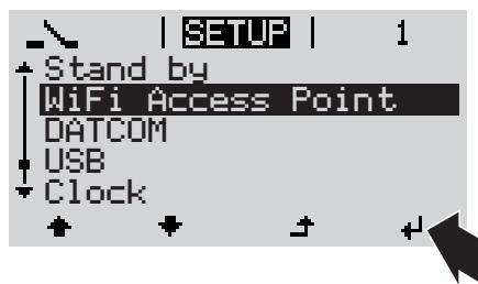
The inverter establishes the WLAN Access Point. The WLAN Access Point stays open for one hour. The IP switch on the Fronius Datamanager 2.0 can remain in switch position B by activating the WLAN Access Point.
