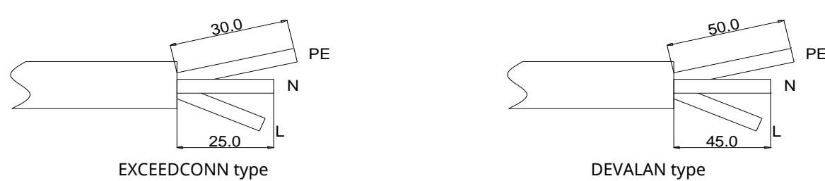
FIG. 7-3 Adjust the Cable Length
