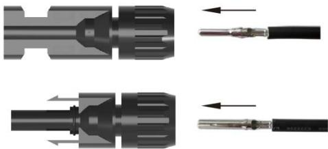
FIG. 7-12 Insert the Contact
