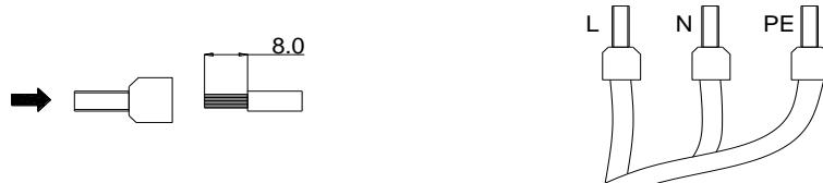
FIG. 7-4 Crimp the Three-core's Ferrule
